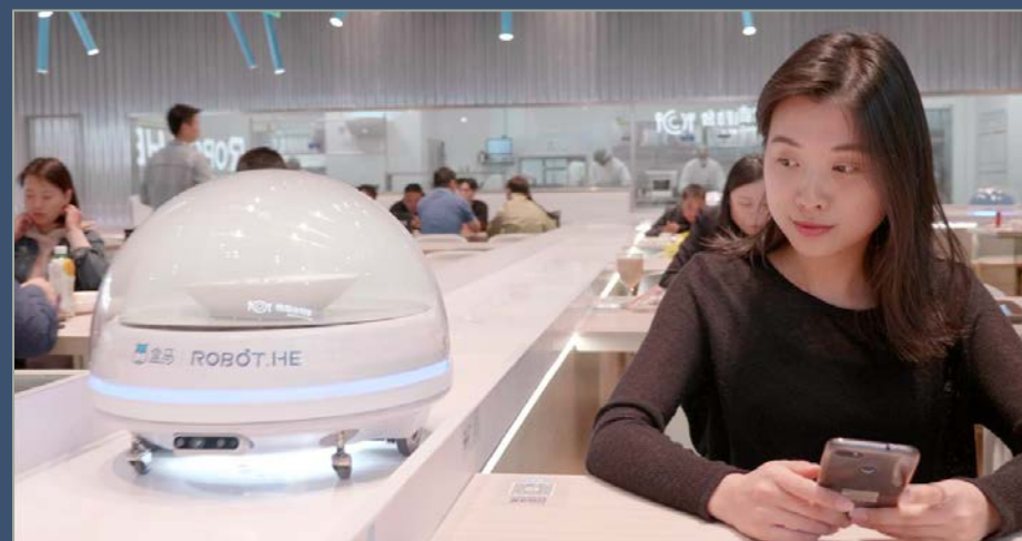
Alibaba's Freshippo restaurant concept is a modern spin on the 'automat' where food was placed in 'lockers' that patrons opened and took their food from. This full-service, robotic version includes a 'runway' that small, wheel robots deliver hot and cold dishes to tables. photo credit: alizila.com
