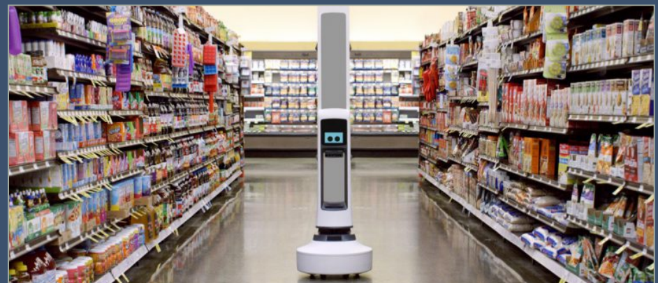
An autonomous UV-equipped disinfecting robot cleaning a grocery store aisle. Average price per robot is around U.S. $125,000. photo credit: Silicon Canals
